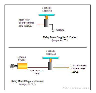
One type of solenoid has only one wire, and is grounded through the case, so it must have the relay board supply 12 volts. You would set the jumper to 'V'. This is the most common option, unless you are converting a previously injected engine which is wired for 'active ground' and you wish to use the existing fast idle valve and wiring (though most EFI engines don't have a FIdle valve, they have a stepper motor, which won't work with MegaSquirt in any case).
