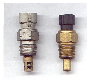
Note that these sensors have different connectors. The coolant temperature sensor uses a "mushroom" shaped key way where it inserts into the sensors, while the open element intake air temperature sensor uses a "rectangular" connector key way.
