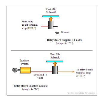
If you are designing you own wiring system and using an 'off-the-shelf' vacuum solenoid with two wires, you can do it either way, so long as the solenoid isn't grounded through the case.
