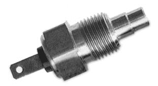
(There is also a spade type GM sensor with a <sup>1</sup>/4" NPT thread available as GM part number **25036292**. This part was originally used as an oil temperature sensor on 84-87 Corvettes, and has the same resistance curve as other GM sensors.)
