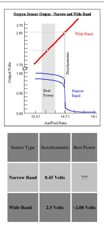
If your car did not come with an oxygen sensor, you can add one. The thread for all oxygen sensors [including wide-band] is: **18mm x1.5mm** - i.e., a metric thread 18mm in diameter with a pitch of 1.5mm, the same as 18mm spark plugs. The hex portion is 22mm, and a 7/8" wrench will work for installing/removing.
