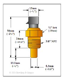
However, you will save some money if you can source these from a salvage yard, with the mating connectors (which are GM #12162193). If you are unable to get them this way, consider using a "spade-type" connector or reusing your existing sensors (with EasyTherm and/or resistor calibration adjustments).
