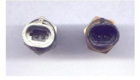
The wiring schematic for DB37 shows only one input for all of the sensors (except for the two for the TPS). The recommended GM sensors all have two wire connectors. The missing connection is a ground wire for the sensor. Sensor grounds should be brought to the same grounding point on the engine block as the MegaSquirt ground, unless they are grounded through the body of the sensor.
