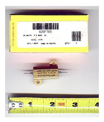
Ohmite has several suitable resistors, with part numbers that start 825F (25 Watt, aluminum case with mounting ears) and end in XRY, where X and Y indicate X.Y ohms. Depending on injector, pick 2-8 ohms or so.
