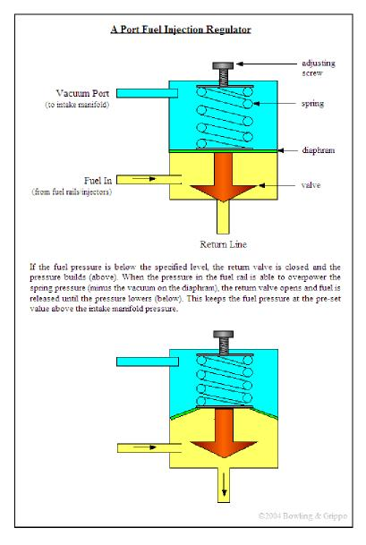
If you are using an aftermarket fuel pressure regulator, it is a good idea to also install a pressure gauge, since most of these are adjustable. For TBI, use a 0-30 psi gauge. For
