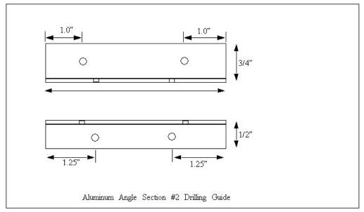
Make sure your heat sink is no longer than  $3\frac{1}{2}$ " (89mm), so that it can sit flat against the case. The edge of the heat sink is flush with the end of the case. Drill corresponding holes in the case. Be sure to drill the correct end of the case (the DB9/LED end). Verify that the heat sink will sit flat when bolted to the case.
