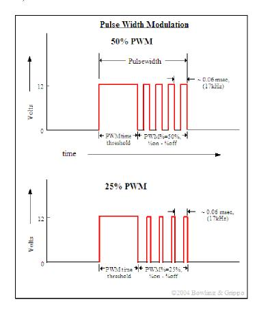
PWM works by switching the 12 volt ground to the injector on and off very rapidly (in about 0.000059 seconds!). The ratio of the "on" time to the "off" time determines the current through the injectors. However, the easiest way to think of the PWM% is as a percentage of the supply voltage, so 50% PWM on a 14 volt supply becomes effectively 7 volts on average, 28% would be 4 volts, etc.
