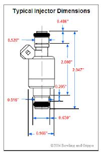
The manifold injector bungs are  $\overline{0.530"-0.535"}$  inside diameter [about 17/32" or 13.5 mm]. The fuel supply rail bungs for the top of the injectors are the same size.
