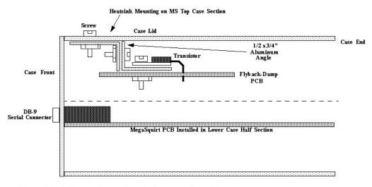
Note: Apply heatsink compound on transistor, aluminum angle, and case lid at all adjoining sections
